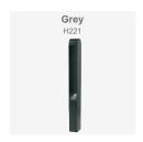
Bollard made of Grey-100 steel treated with Ferrus, a protective process that guarantees high resistance to corrosion. This treatment consists of three layers applied after shot cleaning all impurities: zinc plated, epoxy primer cocating.
